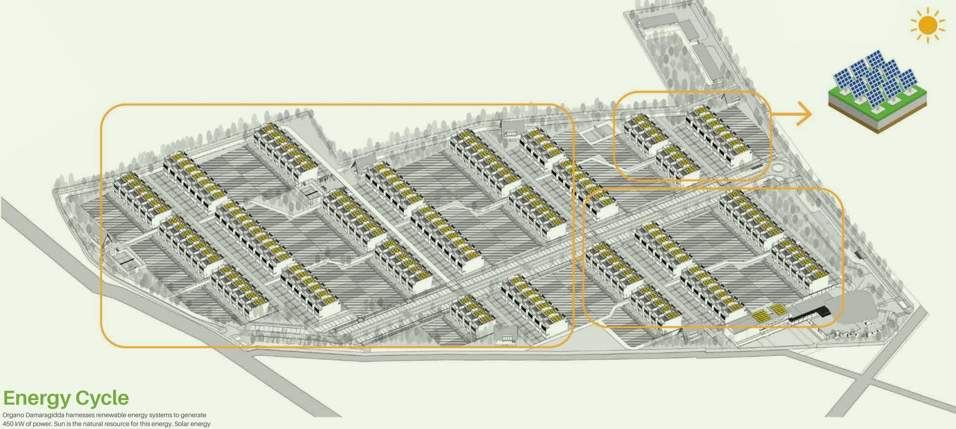
450 kW of power. Sun is the natural resource for this energy. Solar energy is produced and shared between the homes so that any variation in the load will be taken care of by the solar panels. There is an off grid system that is separated from the main government grid. The solar panel is connected to all the appliances. The energy requirement is carefully calculated according to each appliance. Every appliance has an apt location as a part of the unit design.
