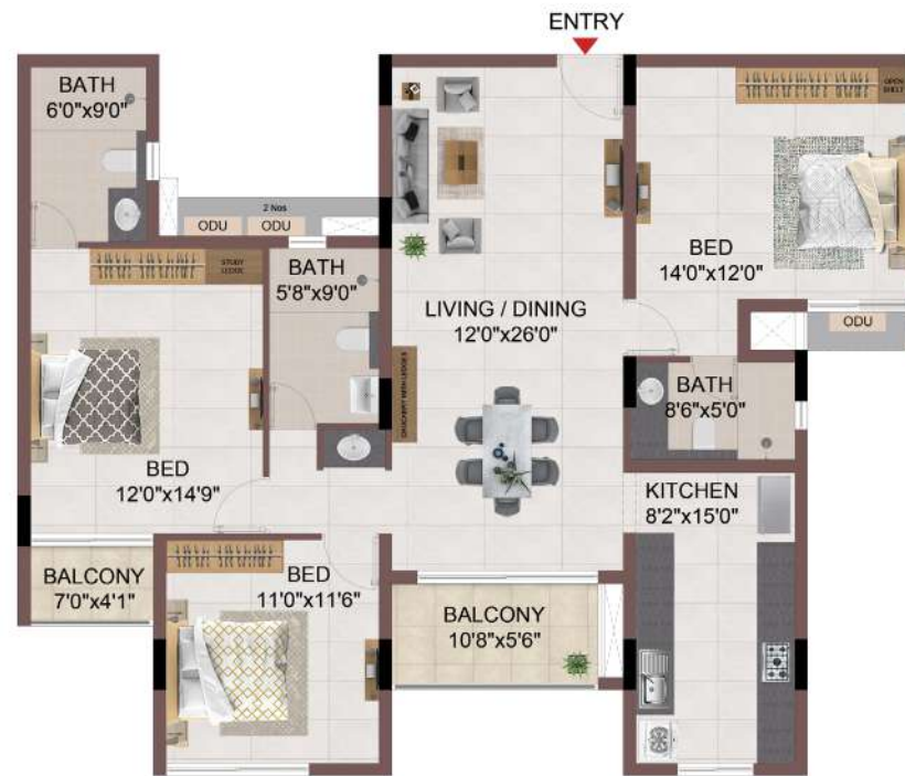
TYPICAL FLOOR 1ST TO 4TH
