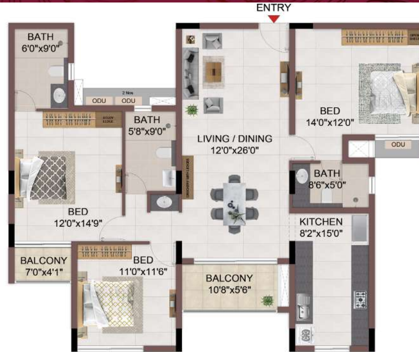
TYPICAL FLOOR 1ST TO 4TH
