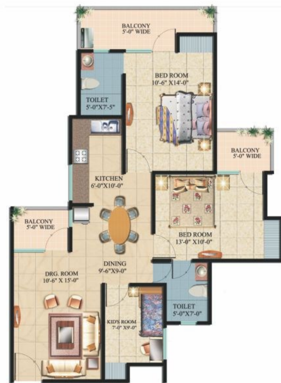
Super Area= 1265 Sq. Ft. 2 Bed Rooms + 2 Toilets + Kid's Room + Drawing / Dining + Kitchen + Balconies + Utility
