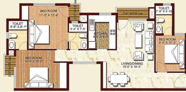
TYPE 4 (3 BHK+ 3T) T. CARPET AREA - 971 SQ.FT. (90.2089 SQ. M.) T. CARPET+ BALCONY AREA - 1038 SQ.FT. (96.43336 SQ. M.) TOWERS - B,C,D,E,F,G,H,I,J
