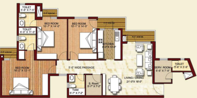
TYPE - 6 (3 BHK+ 3T + STUDY + SERVANT) T. CARPET AREA - 1250 SQ.FT. (116.1288 SQ. M.) T. CARPET+ BALCONY AREA - 1377 SQ.FT. (127.9275 SQ. M.) TOWERS - B,C,D,E,F,G,H,I,J Typical Floor Plan (Ground, 3rd, 4th, 5th, 7th, 8th, 9th, 11th, 12th, 14th, 15th, 17th, 18th)
