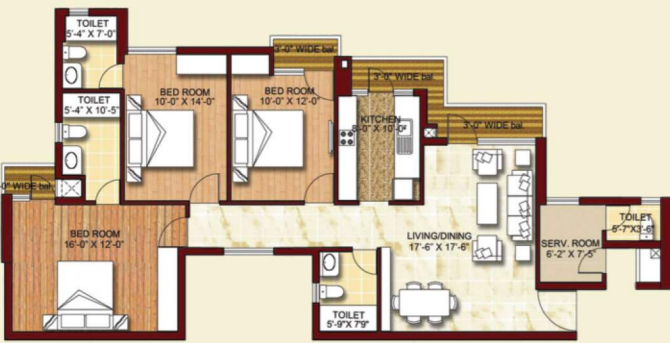
TYPE - 5 (3 BHK+ 3T + SERVANT) T. CARPET AREA - 1137 SQ.FT. (105.6308 SQ. M.) T. CARPET+ BALCONY AREA - 1246 SQ.FT. (115.7572 SQ. M.) TOWERS - B,C,D,E,F,G,H,I,J Typical Floor Plan (Ground, 3rd, 4th, 5th, 7th, 8th, 9th, 11th, 12th, 14th, 15th, 17th, 18th)
