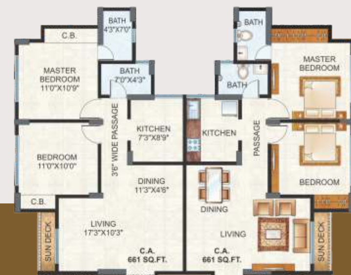
'C2' BUILDING TYPICAL FLOOR PLAN PHASE III
