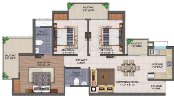
1340 SQ.FT 3 BHK + 2 TOILET SUPER AREA = 1340 SQ. FT. CARPET AREA = 768 SQ. FT. (TOWER C&D)
