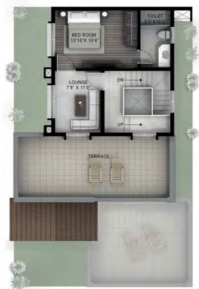
STAIRCASE ROOM FLOOR PLAN
