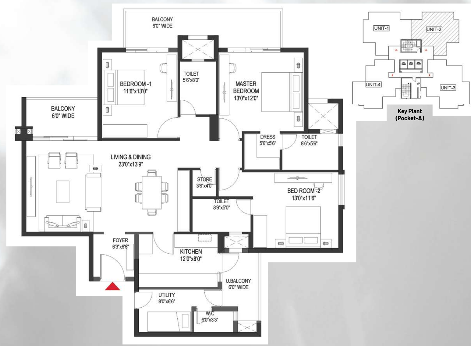
LAYOUT PLAN UNIT-2 14TH TO 27TH FLOOR PLAN 3BHK + UTILITY
