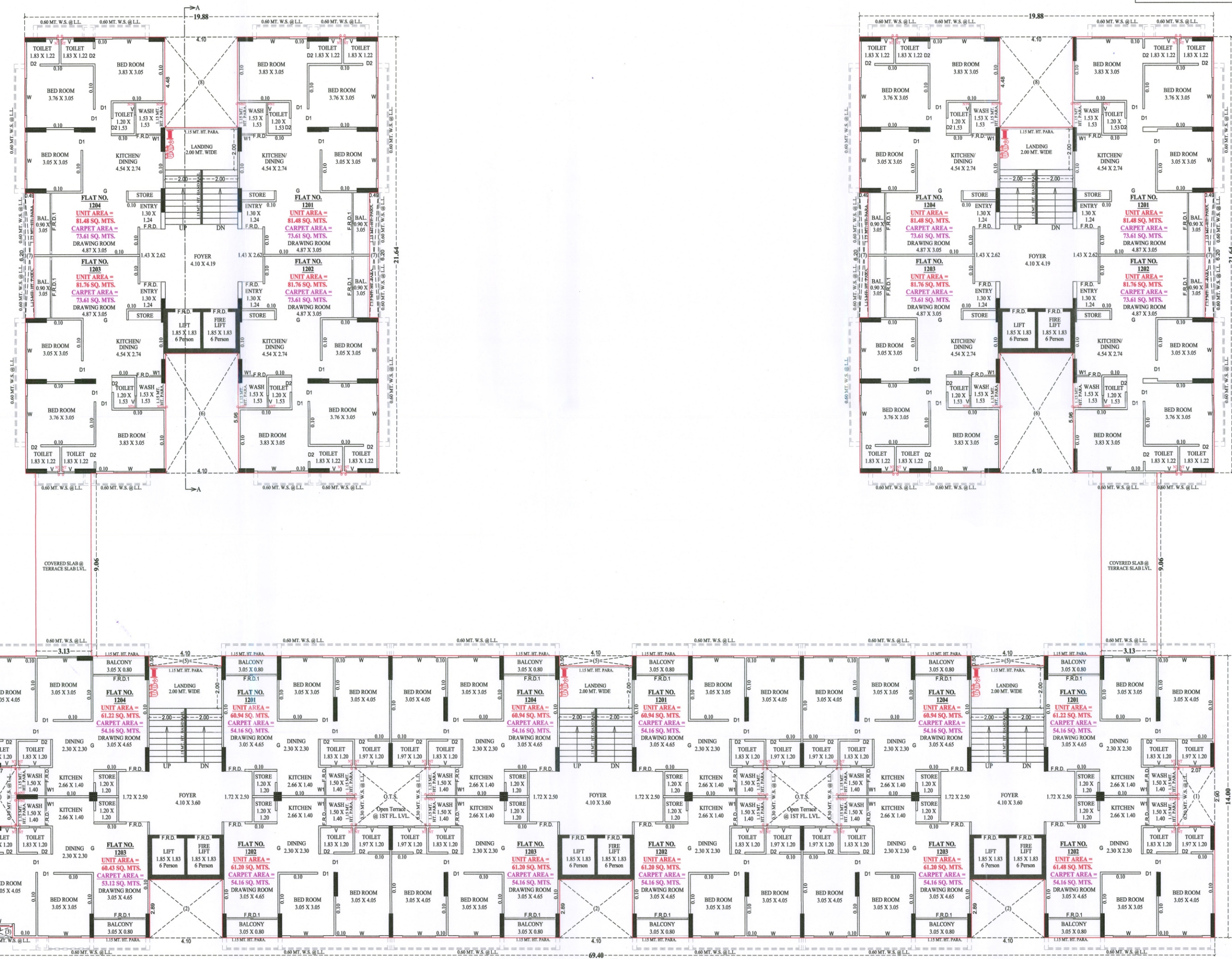
12TH FLOOR PLAN NOTE - ALL OUTER & INTERNAL WALL ARE OF 0.115MT. TH. BK WALL
