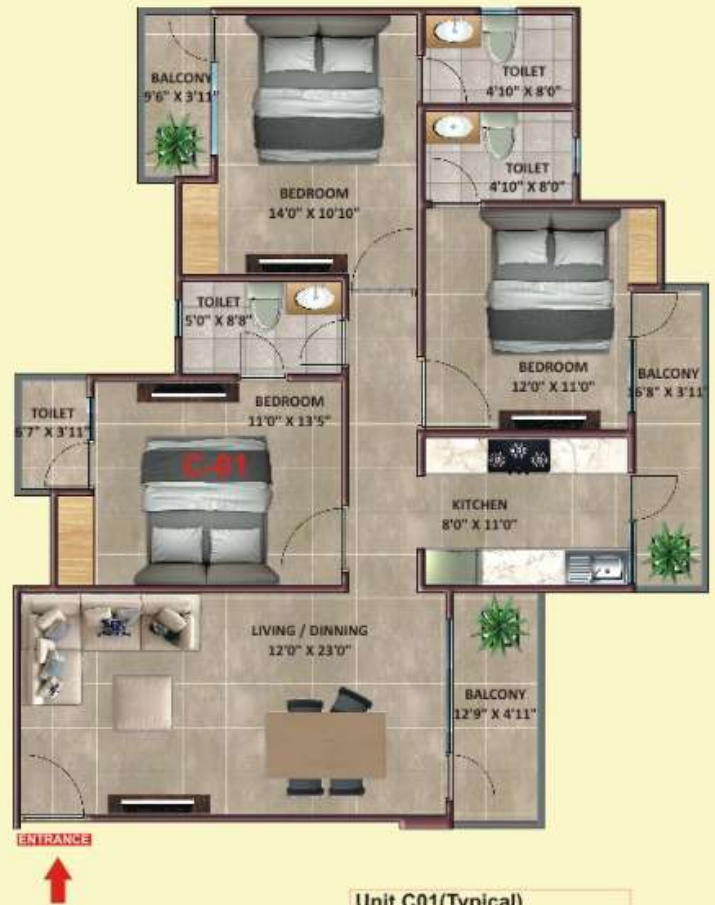
Unit C01 (Typical) Built Up Area = 1298.03 sq. ft. Super Area = 1583.59 sq. ft. Carpet Area = 1005.57 sq. ft.
