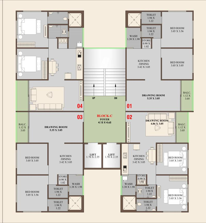
BLOCK - C 1ST TO 13TH FLOOR PLAN
