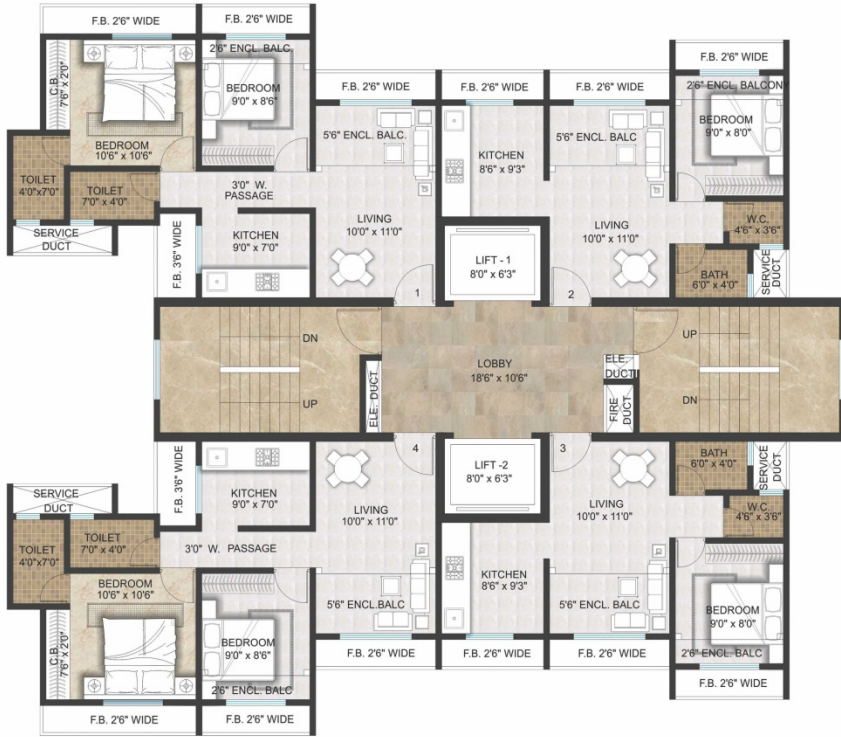
PROPOSED TYPICAL FLOOR PLAN BLDG - A1 (3rd Floor to 18th Floor) REFUGE AREA - 7th, 12th, 17th Floor FLAT NO. 703, 1203, 1703
