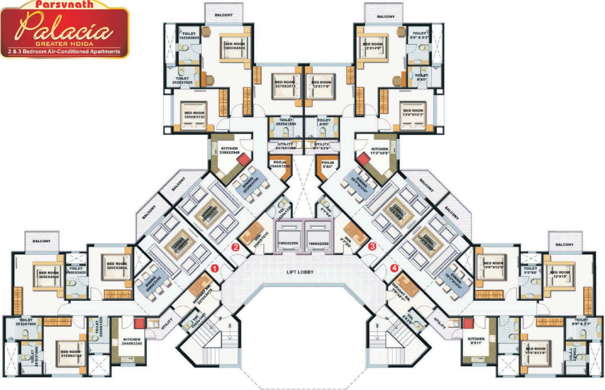
TYPICAL FLOOR PLAN Tower No. A1, A2, A3 & A4 Accomodation : 3 Bedroom + Servant Area : 1835 sq. ft.
